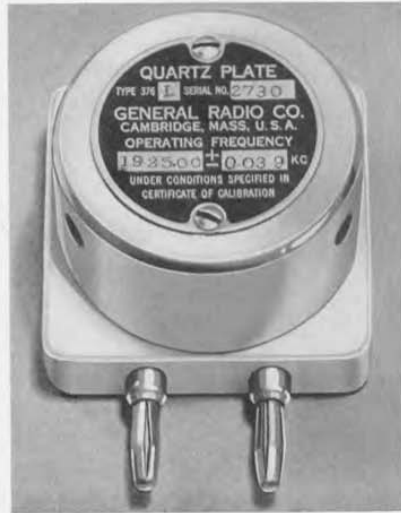
FIGURE 1 (above). External view of holder used for TYPE 376-L Quartz Plates
